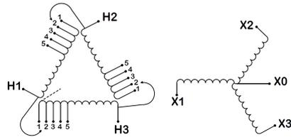
Three Phase Isolation Transformer with a capacity of 45kVA, transforming 240 Volts to 230Y/133 Volts
