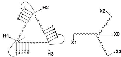
Three Phase Isolation Transformer with a capacity of 45kVA, transforming 240 Volts to 220Y/127 Volts
