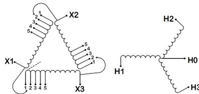
Three Phase Isolation Transformer with a capacity of 45kVA, transforming 208 Volts to 230Y/133 Volts
