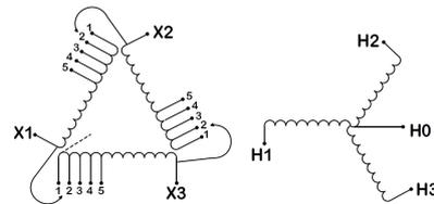
Three Phase Isolation Transformer with a capacity of 45kVA, transforming 200 Volts to 575Y/332 Volts
