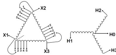
Three Phase Isolation Transformer with a capacity of 45kVA, transforming 120 Volts to 600Y/347 Volts
