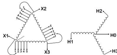
Three Phase Isolation Transformer with a capacity of 45kVA, transforming 120 Volts to 575Y/332 Volts
