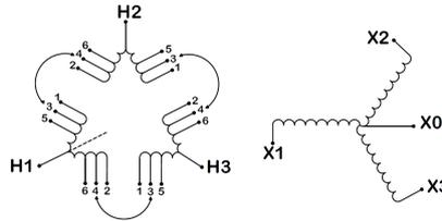
Three Phase Isolation Transformer with a capacity of 450kVA, transforming 575 Volts to 460Y/266 Volts
