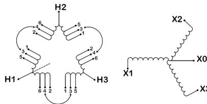
Three Phase Isolation Transformer with a capacity of 450kVA, transforming 550 Volts to 460Y/266 Volts
