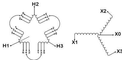
Three Phase Isolation Transformer with a capacity of 450kVA, transforming 440 Volts to 208Y/120 Volts
