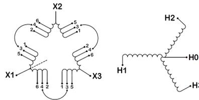
Three Phase Isolation Transformer with a capacity of 450kVA, transforming 220 Volts to 440Y/254 Volts
