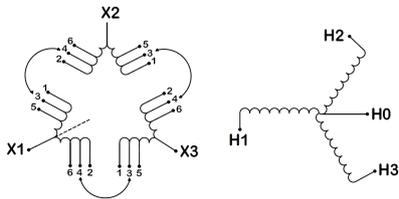
Three Phase Isolation Transformer with a capacity of 450kVA, transforming 120 Volts to 400Y/231 Volts
