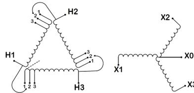
Three Phase Isolation Transformer with a capacity of 3kVA, transforming 277 Volts to 230Y/133 Volts
