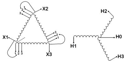
Three Phase Isolation Transformer with a capacity of 3kVA, transforming 120 Volts to 480Y/277 Volts
