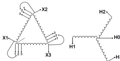
Three Phase Isolation Transformer with a capacity of 3kVA, transforming 110 Volts to 230Y/133 Volts
