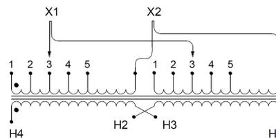
Single Phase Isolation Transformer with a capacity of 37.5kVA, transforming 110 Volts to 120/240 Volts
