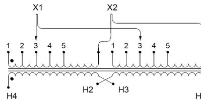
Single Phase Isolation Transformer with a capacity of 330kVA, transforming 440 Volts to 440 Volts
