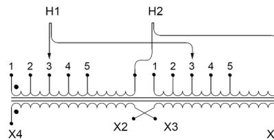
Single Phase Isolation Transformer with a capacity of 330kVA, transforming 416 Volts to 347 Volts
