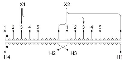
Single Phase Isolation Transformer with a capacity of 330kVA, transforming 240 Volts to 400 Volts
