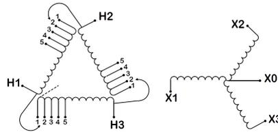
Three Phase Isolation Transformer with a capacity of 30kVA, transforming 575 Volts to 550Y/318 Volts
