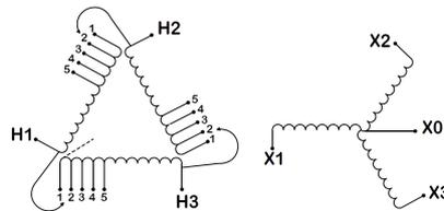
Three Phase Isolation Transformer with a capacity of 30kVA, transforming 575 Volts to 380Y/220 Volts
