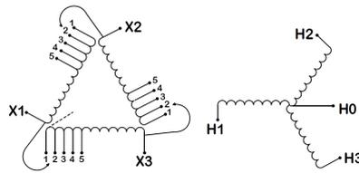
Three Phase Isolation Transformer with a capacity of 30kVA, transforming 208 Volts to 380Y/220 Volts
