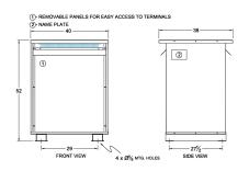
Three Phase Isolation Transformer with a capacity of 300kVA, transforming 380 Volts to 220Y/127 Volts
