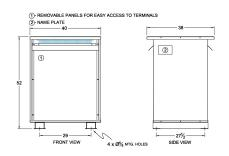
Three Phase Isolation Transformer with a capacity of 300kVA, transforming 347 Volts to 480Y/277 Volts
