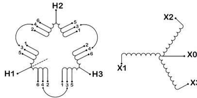
Three Phase Isolation Transformer with a capacity of 300kVA, transforming 600 Volts to 550Y/318 Volts
