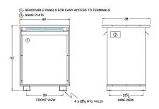
Three Phase Isolation Transformer with a capacity of 300kVA, transforming 575 Volts to 220Y/127 Volts
