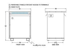
Three Phase Isolation Transformer with a capacity of 300kVA, transforming 208 Volts to 440Y/254 Volts
