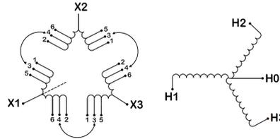
Three Phase Isolation Transformer with a capacity of 300kVA, transforming 115 Volts to 208Y/120 Volts
