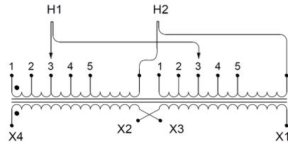
Single Phase Isolation Transformer with a capacity of 250kVA, transforming 480 Volts to 230/460 Volts
