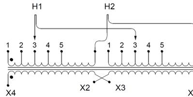
Single Phase Isolation Transformer with a capacity of 250kVA, transforming 230 Volts to 115/230 Volts
