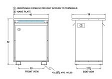
Three Phase Isolation Transformer with a capacity of 225kVA, transforming 480 Volts to 550Y/318 Volts
