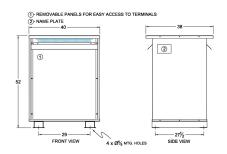
Three Phase Isolation Transformer with a capacity of 225kVA, transforming 460 Volts to 480Y/277 Volts
