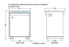
Three Phase Isolation Transformer with a capacity of 225kVA, transforming 415 Volts to 440Y/254 Volts
