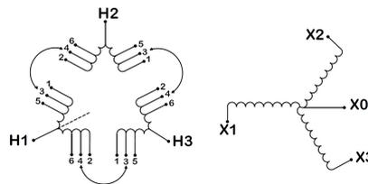
Three Phase Isolation Transformer with a capacity of 225kVA, transforming 550 Volts to 380Y/220 Volts
