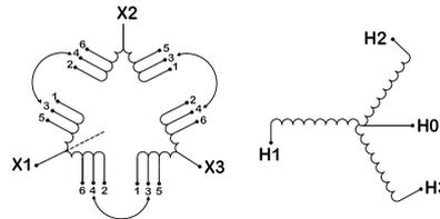
Three Phase Isolation Transformer with a capacity of 225kVA, transforming 380 Volts to 440Y/254 Volts
