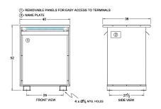
Three Phase Isolation Transformer with a capacity of 225kVA, transforming 347 Volts to 240Y/139 Volts
