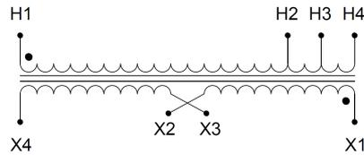
Single Phase Isolation Transformer with a capacity of 1kVA, transforming 600 Volts to 120/240 Volts
