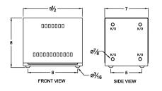
Single Phase Isolation Transformer with a capacity of 1kVA, transforming 110 Volts to 110/220 Volts
