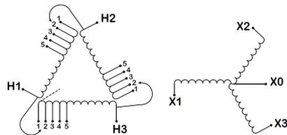
Three Phase Isolation Transformer with a capacity of 15kVA, transforming 600 Volts to 550Y/318 Volts
