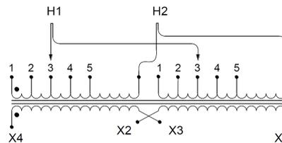
Single Phase Isolation Transformer with a capacity of 15kVA, transforming 575 Volts to 480 Volts
