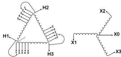
Three Phase Isolation Transformer with a capacity of 15kVA, transforming 480 Volts to 460Y/266 Volts
