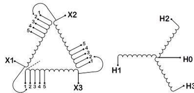
Three Phase Isolation Transformer with a capacity of 15kVA, transforming 400 Volts to 440Y/254 Volts
