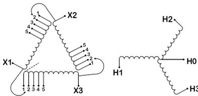
Three Phase Isolation Transformer with a capacity of 15kVA, transforming 380 Volts to 415Y/240 Volts
