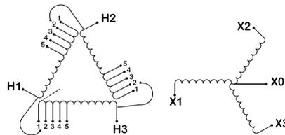
Three Phase Isolation Transformer with a capacity of 15kVA, transforming 277 Volts to 240Y/139 Volts
