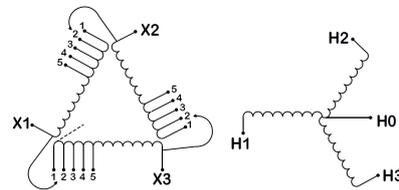
Three Phase Isolation Transformer with a capacity of 15kVA, transforming 208 Volts to 380Y/220 Volts
