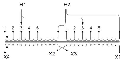
Single Phase Isolation Transformer with a capacity of 15kVA, transforming 200 Volts to 120/240 Volts
