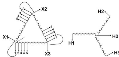
Three Phase Isolation Transformer with a capacity of 15kVA, transforming 120 Volts to 416Y/240 Volts
