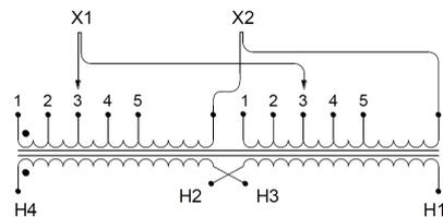
Single Phase Isolation Transformer with a capacity of 15kVA, transforming 115 Volts to 440 Volts
