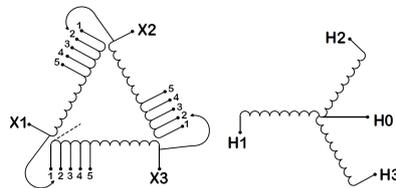
Three Phase Isolation Transformer with a capacity of 150kVA, transforming 220 Volts to 416Y/240 Volts
