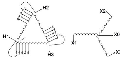
Three Phase Isolation Transformer with a capacity of 112.5kVA, transforming 600 Volts to 230Y/133 Volts
