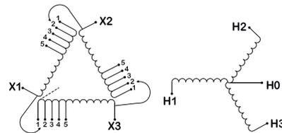
Three Phase Isolation Transformer with a capacity of 112.5kVA, transforming 110 Volts to 550Y/318 Volts
